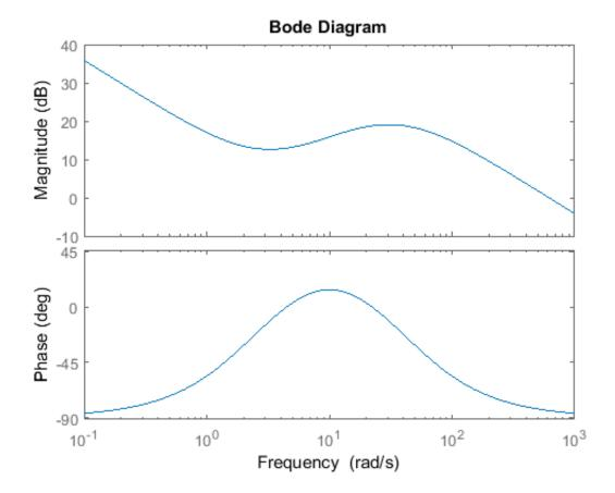
Closed-loop stability We can verify that the final controller K4 results in closed-loop stability. Formally we need to check the stability of all closed-loop transfer functions. For simplicity, we'll check the poles of the complementary sensitivity function. This closed-loop transfer function has all poles in the left half of the complex plane and hence it is stable.
