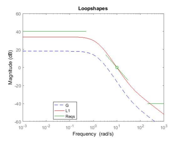
Phase Margin for L1 The MARGIN command can be used to compute the gain and phase margins for a system. This command shows that L1 has 31degs of phase margin at the cross-over frequency. This confirms that L1 does not satisfy the robustness requirement (R5).
