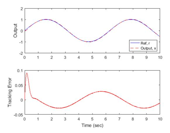
Linear Analysis The simulation results can be verified using frequency response analysis. In the Laplace domain the output is related to the reference command and noise by: X(s) = T(s)\*R(s) - T(s)\*N(s) where T is the complementary sensitivity function. For linear systems, these two effects add linearly and we can analyze them separately.
