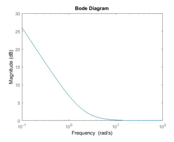
Bode plot of loopshape L2 with requirements L2 now satisfies tracking requirement (R3) and crossover requirement (R2). It does not satisfy the noise rejection (R5) and robustness requirements (R5). Also, notice that the loopshape L2 is very similar to the loopshape L1 at high frequencies. The integral boost has increased the low frequency gain with small effect at higher frequencies.
