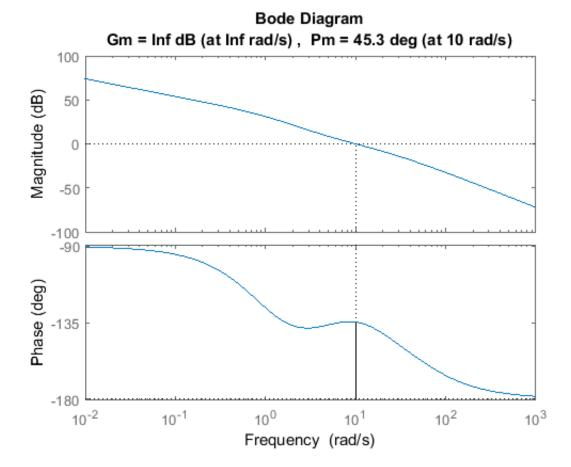
Bode plot of loopshape L4 with requirements L4 now satisfies the robustness margin requirement. However, the lead controller has decreased the low frequency gain. As a result L4 slightly violates the low frequency tracking requirement (R3). We can go back and iterate on our various choices to ensure that all requirements are satisfied. However, we'll go ahead with this design since it almost satisfies all requirements.
