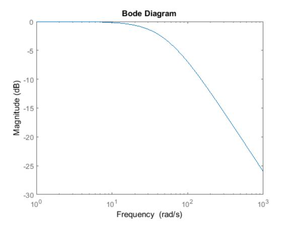
Bode plot of loopshape L3 with requirements L3 now satisfies all requirements except the robustness requirement (R5). Also, notice that the loopshape L3 is very similar to the loopshape L2 at low frequencies. The roll-off decreases the high frequency gain with small effect at lower frequencies.
