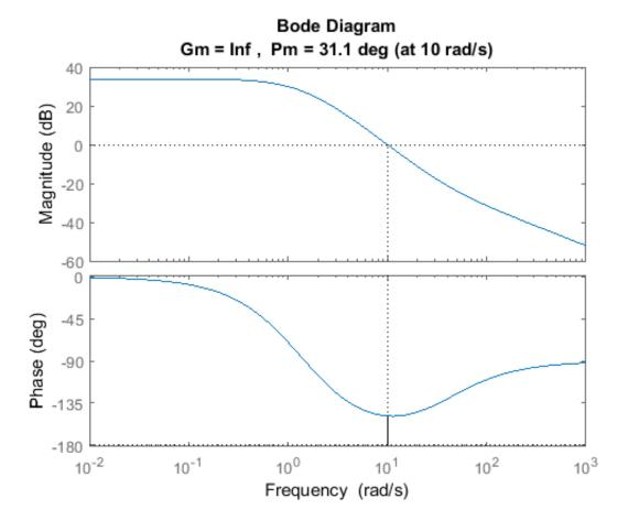
Unit Step Response The original plant G has a gain crossover at w=3.7rad/sec. The loopshape L1 has a gain crossover at w=10rads/sec. Thus we expect L1 to have a faster **closed-loop** response than G because it has a higher **open-loop** crossover frequency. The step responses show that the closed-loop with L1 has a faster rise time and settling time. However, the response with L1 has a larger overshoot. The large overshoot is related to the small phase margin achieved by L1.
