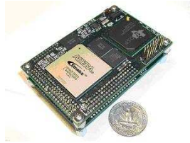
Figure. 7. FCS20 custom flight computer
