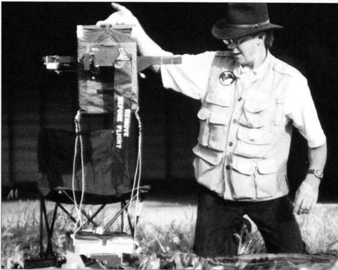
The author lifting the module of one of his near spacecraft. The second module is green and can partially be seen in the grass. The "Remove Before Flight" tag is a reminder for launch crews to open the camera before launching the mission. (Photo courtesy of Shari Conner, K9XTN)
