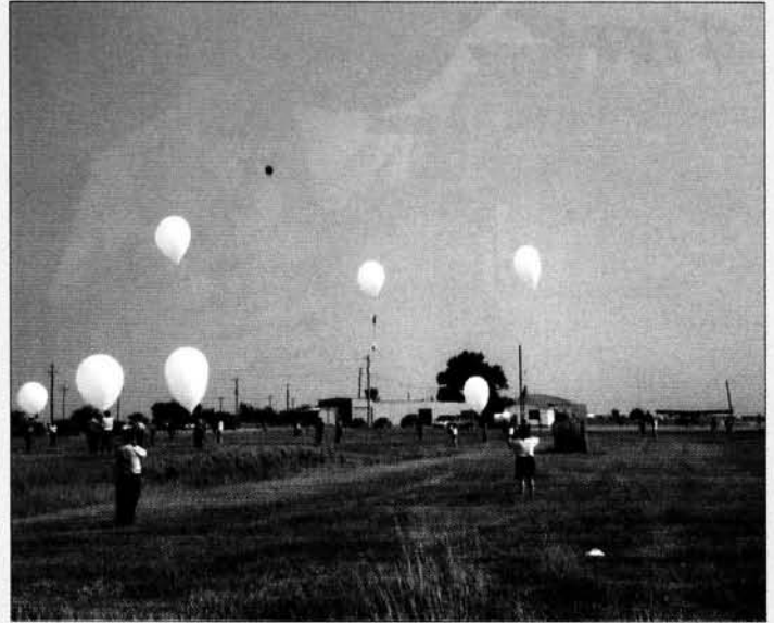
Six stacks are about to be launched. You'll actually count eight balloons because of the red piball (pilot balloon) and the extra balloon on Don Pfister's stack. The piball was launched by EOSS to gauge wind speed and direction before GPSL 2002 launched.
