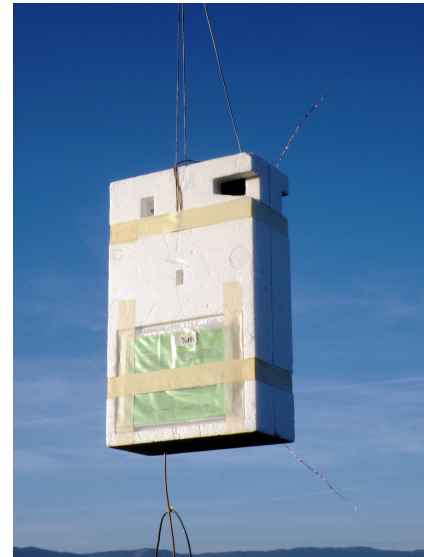
Figure 13. Meteolabor SRS-C34 radiosonde with original thermocouple temperature sensor fixed to thin wires that extend at a 45° angle upward (above right) and an additional thermocouple temperature sensor at a 45° angle downward (below right).
