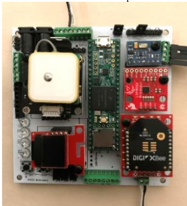
A populated, and wired, PTERODACTYL. The pair of wires at the top go to an external on and off switch. The pair of wires at the bottom go to the PTERODACTYL external thermistor. The four wires on the right (Ground/black, 3.3V/red, SCL/yellow, SDA/blue) go to the IR camera.
