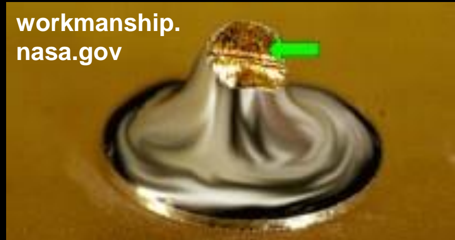
Example of a good solder filet
