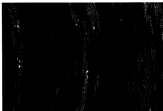
FIGURE 11. Rings give way to wider and shorter aggregates after 2 min of stronger shear at \Omega = 15.7 r.p.m.
