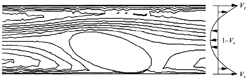
FIGURE 13. Streamlines around the capsule in steady flying. Re = 1000 , \rho = 1.02 , time step = 460, t = 97.23 .
