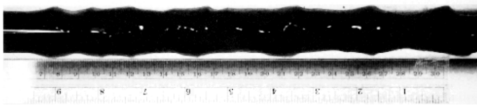
Figure 5: The saw-tooth waves on the oil core in a horizontal pipeline. The flow is from left to right.
