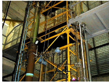
Figure A.3. Vertical flow loop in Venezuela laboratory. 65 ft. long, annulus I.D. 3", internal rod 1". QL = 30-4000 BPD, QG = 1.2-1200 MSCF/D. \mu_0 = 134, 481, 754, 1180 cp. Fully transparent test section, fully instrumented and advance Scada.
