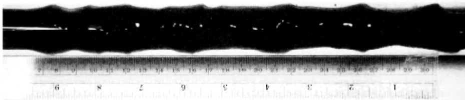
Figure 16. (Joseph, 1997). Core annular flow of #6 fuel. The saw-tooth waves on the oil core in a horizontal pipeline. The flow is from left to right.
