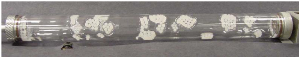
Figure 14. Clustering of particles due to capillarity. The liquid is glycerin with a density of 1.173 g/cm 3 , and the particles are nylon particles with a density of 1.170 g/cm 3 and a diameter of 0.314cm. The
