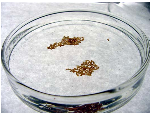
Figure 4. Free motions leading to self-assembly of floating particles. The particles are AcFrac sands with a density of 1.64 \text{ g/cm}^3 and the liquid is a 1% aqueous Polyox solution with a density of 1.006 \text{ g/cm}^3 (see table A1 and A2 in the appendix for more particle and liquid properties). The particles are hydrophobic and are not wetted by the aqueous Polyox solution; the capillary force not only helps the heavier-than-liquid particles float but also draws particles together.
