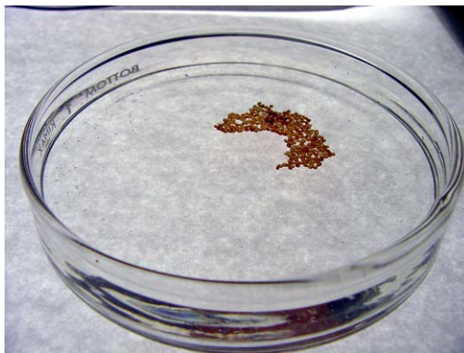
Figure 4. Free motions leading to self-assembly of floating particles. The particles are AcFrac sands with a density of 1.64 \text{ g/cm}^3 and the liquid is a 1% aqueous Polyox solution with a density of 1.006 \text{ g/cm}^3 (see table A1 and A2 in the appendix for more particle and liquid properties). The particles are hydrophobic and are not wetted by the aqueous Polyox solution; the capillary force not only helps the heavier-than-liquid particles float but also draws particles together.
