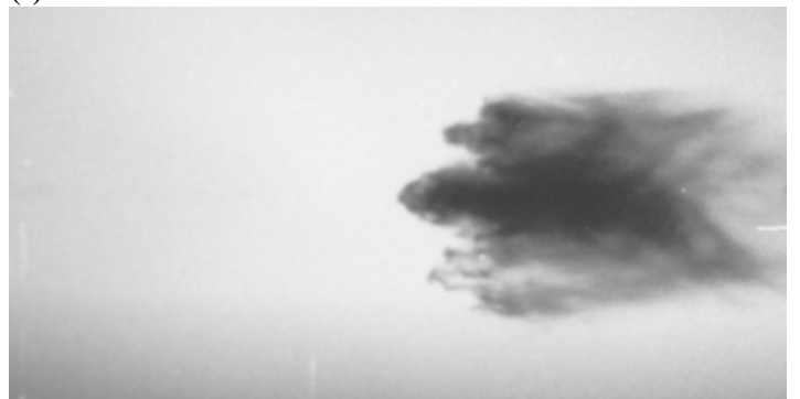
Figure 8. Stages in the breakup of a drop of glycerine (diameter = 2.4 mm ) in the flow behind a Mach 3 shock wave. Air velocity = 758 m/sec; dynamic pressure = 554.0 kPa; Weber no. = 42,200 Time (microseconds): (a) 0 (b) 35 (c) 50 (d) 70 (e) 90 (f) 125 (g) 150 (h) 185
