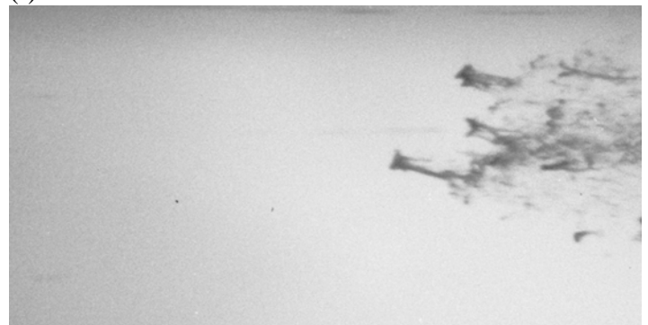
Figure 12. Stages in the breakup of a drop of 2.6% solution of polystyrene butylacrylate (47025-24) in tributyl phosphate (PSBA/TBP ; diameter = 2.2 mm ) in the flow behind a Mach 3 shock wave. Air velocity = 736 m/sec; dynamic pressure = 513.0 kPa; Weber no. = 107,500 Time (microseconds): (a) 0 (b) 30 (c) 50 (d) 80 (e) 105 (f) 135 (g) 160 (h) 200
