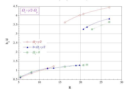
Figure 14. Lift-off of a circular particle from a horizontal wall in a Poiseuille flow of a Newtonian fluid (W/d = 12, l/d = 22,  $\eta$  = 1.0 poise, d = 1 cm,  $\rho_p$  = 1.01 g/cc).
