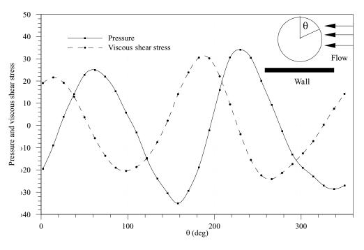
Figure 20(b). Distributions of pressure and viscous shear stress on the surface of a freely rotating circular particle in a Poiseuille flow of a Newtonian fluid. W/d = 12, 1/d = 22, d = 1.0 cm,  $\rho_p/\rho_f = 1.01$ , R = 27 (after bifurcation).
