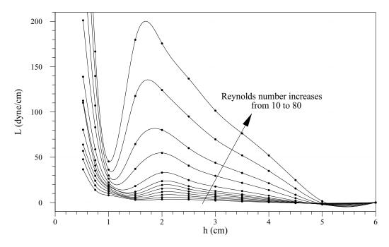
Figure 22. The hydrodynamic lift force on the particle as a function of the height of its center from the bottom wall at different shear Reynolds numbers. The bottom wall is h = 0 cm and the channel centerline is h = 6 cm.
