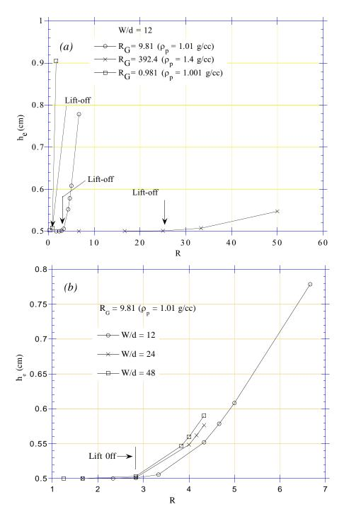
Figure 10. (a) Lift-off and equilibrium height as a function of the shear Reynolds number at different values of  $R_G$ . (b) Equilibrium height vs. shear Reynolds number at different channel widths.
