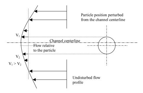
Figure 26. Cartoon showing the fluid velocity relative to a non-rotating particle perturbed from the channel centerline in a plane Poiseuille flow.
