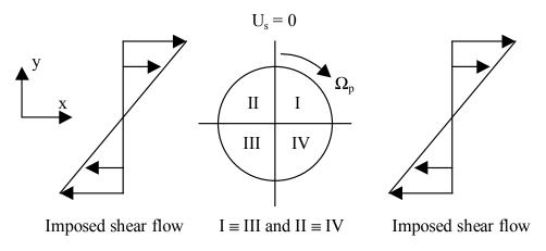
Figure 4. A neutrally buoyant particle in an unbounded linear shear flow.
