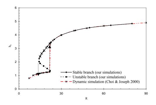
Figure 24. Equilibrium height as a function of shear Reynolds number for a particle of density 1.01 g/cm<sup>3</sup>
