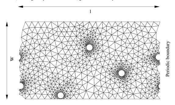
Figure 2. Unstructured mesh in a periodic domain with many particles. In our simulations there is one particle in the domain.
