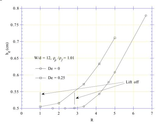
Figure 27. Equilibrium height vs. shear Reynolds number for a particle in a Poiseuille flow of an Oldroyd-B fluid.
