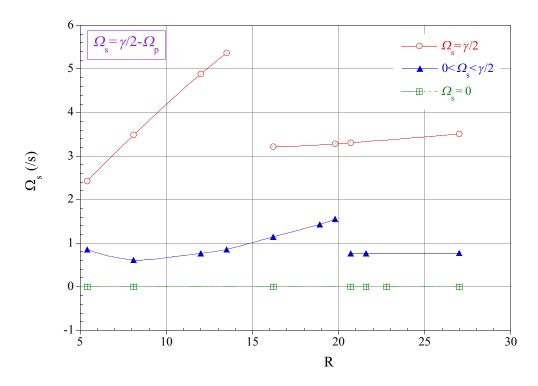
Figure 16. Slip angular velocity vs. shear Reynolds number for the cases depicted in figure 14.
