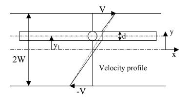
Figure 8. A long rectangular particle in a steady Couette flow. The dotted line represents the undisturbed velocity profile whereas the solid line represents the velocity profile in the presence of the long particle.
