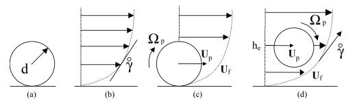
Figure 3. Lift-off and levitation to equilibrium.
