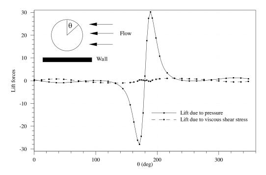
Figure 30(c). The distribution of lift forces on the surface of a freely rotating particle. W/d = 12, l/d = 22, d = 1.0 cm,  $\rho_p/\rho_f$  = 1.001, R = 0.6, Newtonian fluid. The particle does not lift off.
