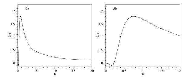
Figure 5. Graphs of  $J(\epsilon)/\epsilon$  vs.  $\epsilon$  for  $\epsilon > 0.025$ . The graphs are based on McLaughlin's data for the lift on a sphere in an unbounded linear shear flow.
