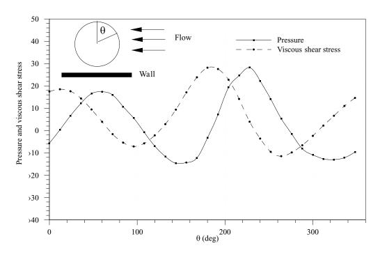
Figure 20(e). Distributions of pressure and viscous shear stress on the surface of a non-rotating circular particle in a Poiseuille flow of a Newtonian fluid. W/d = 12, l/d = 22, d = 1.0 cm,  $\rho_p/\rho_f = 1.01$ , R = 27 (after bifurcation).
