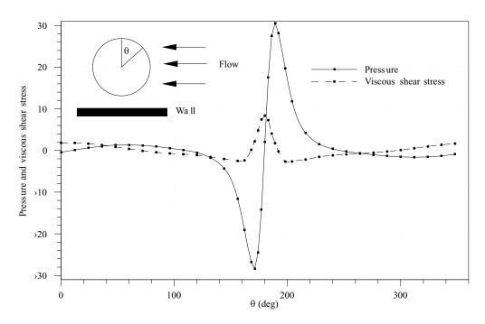
Figure 30(a). Distributions of pressure and viscous shear stress on the surface of a freely rotating circular particle in a Poiseuille flow of a Newtonian fluid. W/d = 12, 1/d = 22, d = 1.0 cm,  $\rho_p/\rho_f = 1.001$ , R = 0.6. The particle does not lift off.
