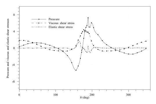
Figure 30(e). Distributions of pressure and viscous and elastic shear stresses on the surface of a lifted circular particle in a Poiseuille flow of an Oldroyd-B fluid. W/d = 12,
