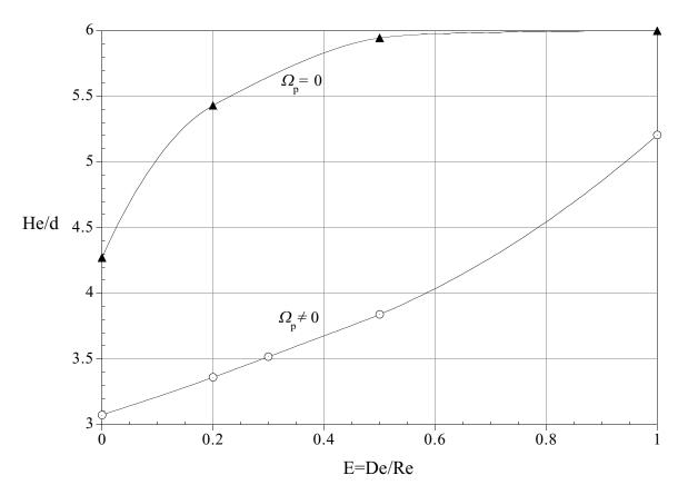
Figure 25. Lift-off of a circular particle from a horizontal wall in a Poiseuille flow of an Oldroyd-B fluid (W/d = 12, l/d = 22,  $\eta$  = 1.0 poise, d = 1.0 cm, R = 0.60).
