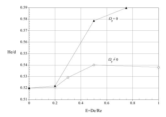
Figure 28. Lift-ff of a circular particle from a horizontal wall in a Poiseuille flow of an Oldroyd-B fluid (W/d = 12, V/d = 22,  $\eta = 1.0$  poise, d = 1.0 cm,  $\rho_p = 1.001$  g/cc).
