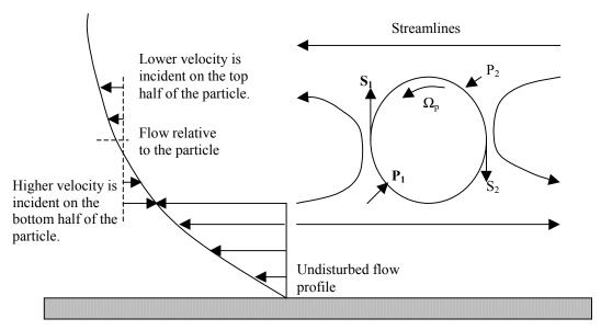
Figure 21. Cartoon depicting the fluid velocity and the streamlines relative to a particle in a plane Poiseuille flow. The fluid approaches the particle with higher velocity in the bottom half of the particle. Consequently, the pressure  $P_1$  (in bold) is greater than  $P_2$  and the viscous shear stress  $S_1$  (in bold) is greater than  $S_2$ .
