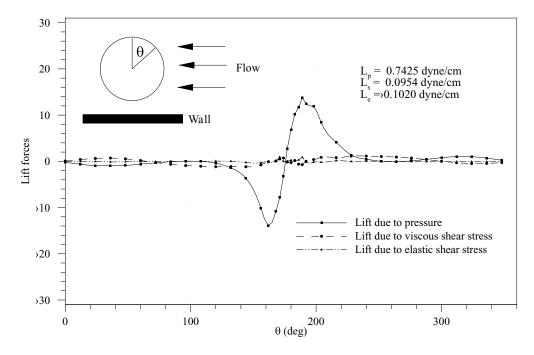
Figure 30(d). The distribution of lift forces on the surface of a freely rotating particle. W/d = 12, 1/d = 22, d = 1.0 cm,  $\rho_p/\rho_f = 1.001$ , R = 0.6, E = 0.5. The particle lifts off.
