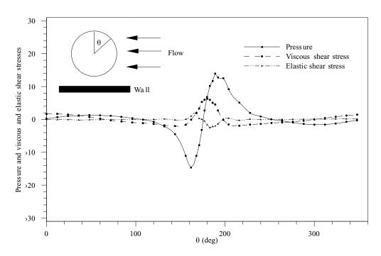
Figure 30(b). Distributions of pressure and viscous and elastic shear stresses on the surface of a freely rotating circular particle in a Poiseuille flow of a Oldroyd-B fluid. W/d = 12, I/d = 22, d = 1.0 cm,  $\rho_p/\rho_f = 1.001$ , R = 0.6, E = 0.5. The particle lifts off.
