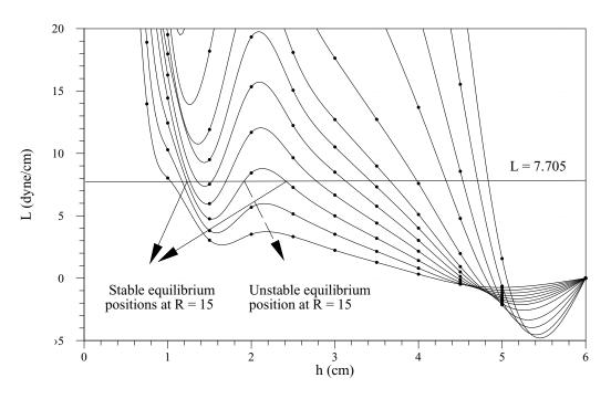
Figure 23. Finding the equilibrium height of a particle of a given density at different values of shear Reynolds number.
