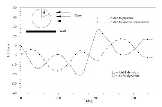
Figure 20(c). The distribution of lift forces on the surface of a freely rotating circular particle in a Poiseuille flow of a Newtonian fluid. W/d = 12, 1/d = 22, 1/d = 10 cm,  $\rho_p/\rho_f = 1.01$ , 1/d = 8.1 (before bifurcation).
