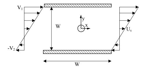
Figure 6. Computational domain for the simulation of linear shear flows around a circular particle.
