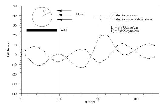
Figure 20(f). The distribution of lift forces on the surface of a non-rotating circular particle in a Poiseuille flow of a Newtonian fluid. W/d = 12, 1/d = 22, 1/d = 10 cm, 1/d = 10, 1/d =
