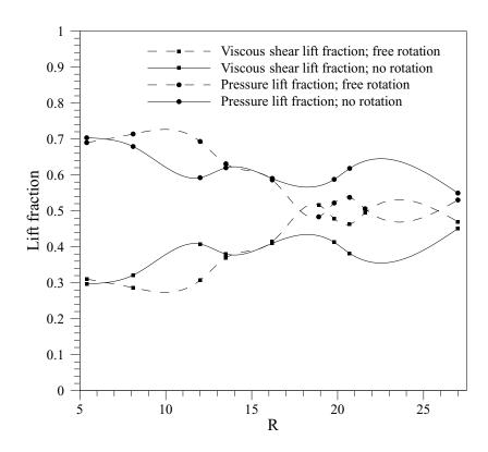
Figure 19. Lift fraction vs. shear Reynolds number for the cases shown in figure 14. Lift fractions for a freely rotating and a non-rotating particle are shown.
