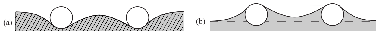
Figure III.3. Spherical particles in water, (a) heavier-than-water hydrophobic particles. The meniscus is below the undisturbed level. If the contact angle doesn't vary the particle must tilt causing an imbalance of the horizontal component of capillary forces pulling the spheres together. Even if the particles do not tilt they will both fall under gravity into the depression between them. (b) Heavier-than-air and lighter-than-water hydrophilic particles. The meniscus is above the undisturbed level. The particle must tilt giving rise to an imbalance of horizontal forces, drawing the particles together. Air bubbles come together.
