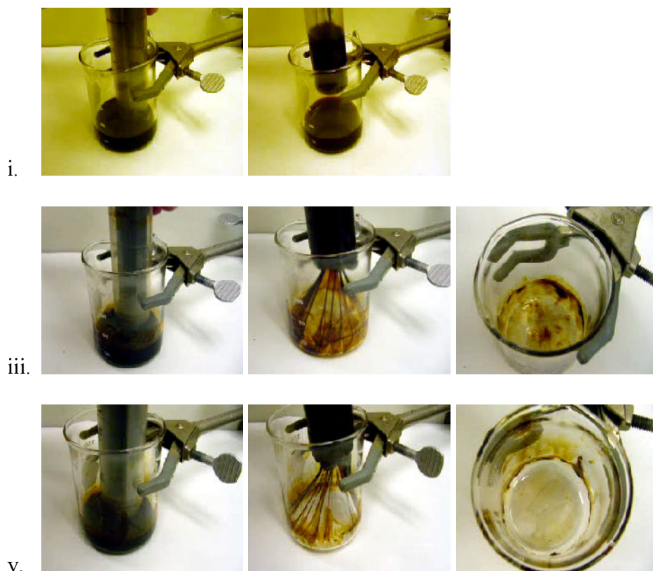
Figure 4. Cleaning oil with Elastol and Elastol plus particles.
