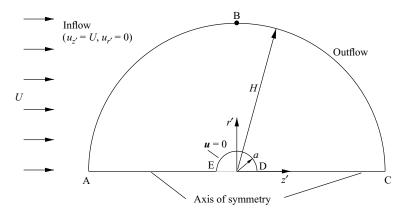
FIGURE 5. Computational domain showing the boundary conditions.
