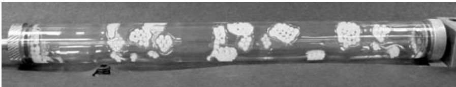
FIGURE 14. Clustering of particles due to capillarity. The liquid is glycerine with a density of 1.173\text{ g cm}^{-3} , and the particles are nylon particles with a density of 1.170\text{ g cm}^{-3} and a diameter of 0.314 cm. The filling level F is 0.082 and the particle concentration is 54.2%. The rotational speed \Omega = 5.45 r.p.m., \beta = 1.127 , average film thickness D_a = 0.585 mm, minimum film thickness D_{min} = 0.526 mm, D_{min}/d_p = 0.176 . Clusters of particles form about 5 min after the beginning of rotation. Bands form occasionally, but are not stable.
