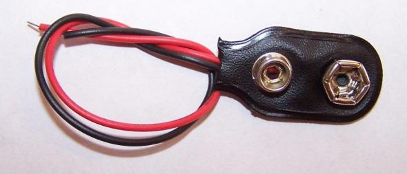
9V battery snap (battery only goes on one way)
