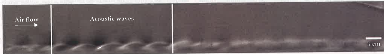
FIGURE 3. ACOUSTIC WAVES in the boundary layer of a Mach 10 flow along the surface of a 1.55-m-long circular cone are evidenced in this Schlieren image. Here, the flow is from left to right, and the image is taken roughly 1.3 m from the tip of the cone. (Image courtesy of Eric Marineau, Air Force Research Laboratory, and Stuart Laurence and Richard Kennedy, University of Maryland.)
