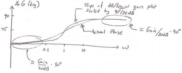
Observation: The net phase change in G from w=0 to w=us is approximately equal to the stope slope of the mignitude curve scaled by  $\frac{95^{\circ}}{200B}$ ,  $\frac{4}{d(161B)} = \frac{90^{\circ}}{200B}$ .  $\frac{d(161B)}{d(165W)} = \frac{90^{\circ}}{100}$  Exact Bode Guis / Phase Formula
